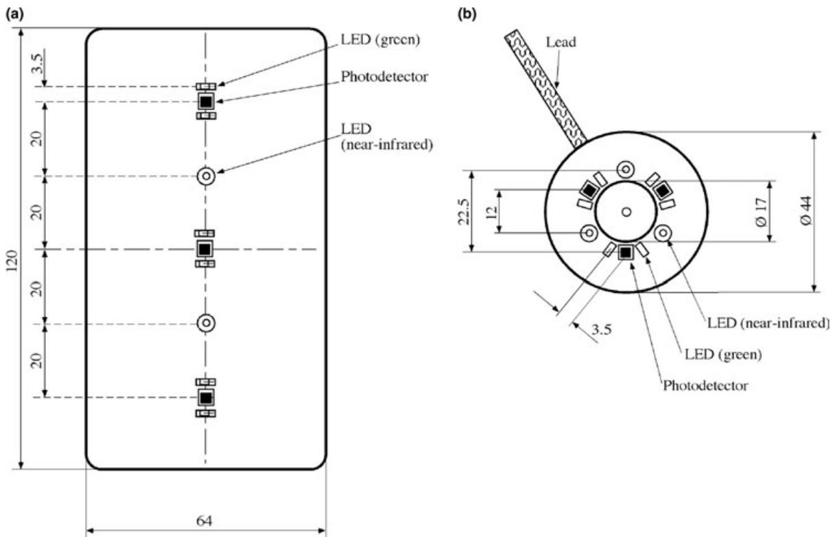
**Figure 2** The rectangular PPG probe (a) and the circular PPG probe (b) used in this study.
