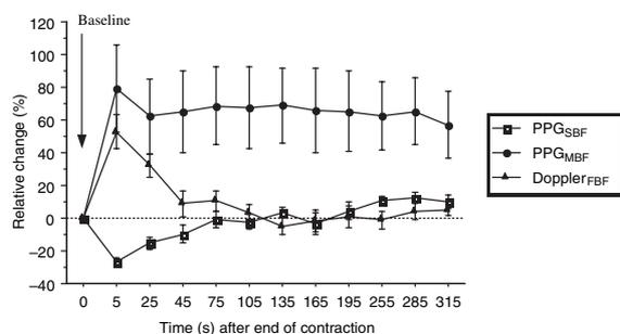
**Figure 7** Relative changes in PPG<sub>SBP</sub> (skin blood perfusion), PPG<sub>MBP</sub> (muscle blood perfusion) and peak Doppler<sub>FBF</sub> (femoral blood flow) at specific time points for 5 min immediately after dynamic contractions. Values (mean  $\pm$  SE) are given as the percentage of the initial resting value (0%).
