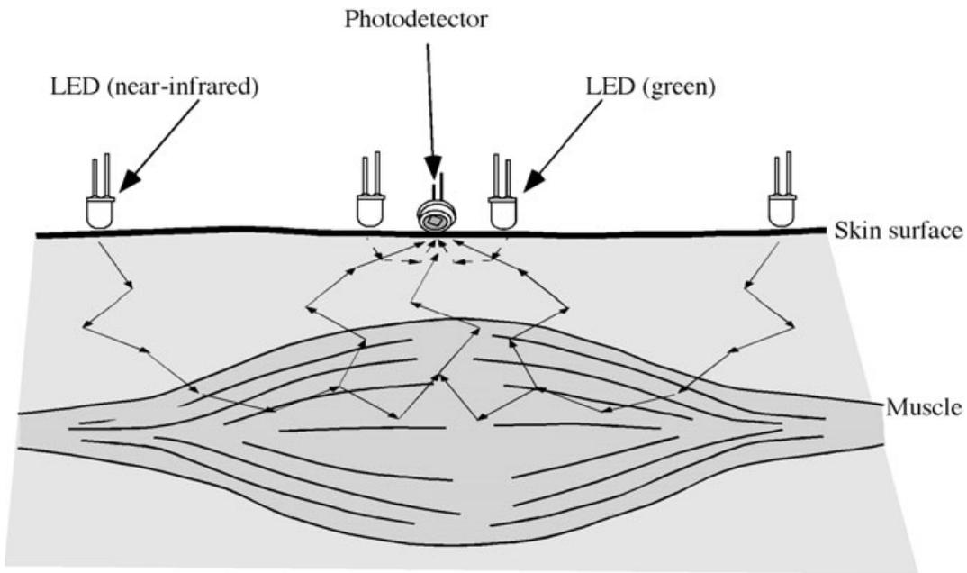
**Figure 1** Schematic description of the photon propagation into tissue emerging from a green light and a near-infrared light source (LED) in combination with different distances between light source and photodetector.
