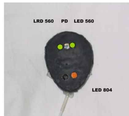
Fig. 4 A PPG probe shown from below including three light-emitting diodes ( LEDs ) and a photodetector ( PD ). The dimensions of the probe are 50 mm×38 mm
